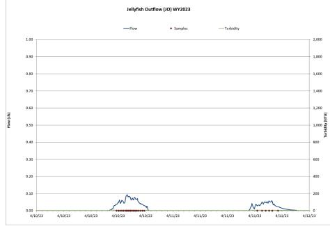
Figure 19 Hydrograph, continuous turbidity, and sample distribution at the Jellyfish Outflow for the 4/10/2023-4/11/2023 non-event snowmelt.
