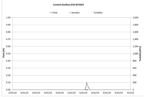
Figure 25 Hydrograph, continuous turbidity, and sample distribution at the Contech Outflow for the 5/31/2023 thunderstorm event.
