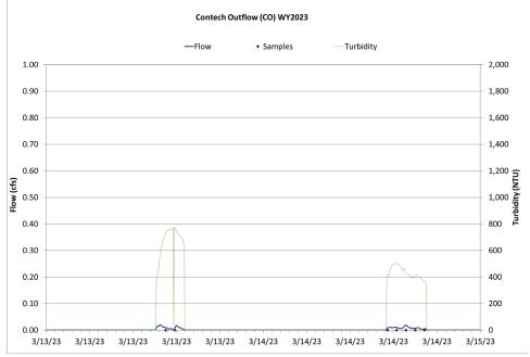
Figure 17 Hydrograph, continuous turbidity, and sample distribution at the Contech Outflow for the 3/13/2023 – 3/14/2023 atmospheric river rain on snow event.
