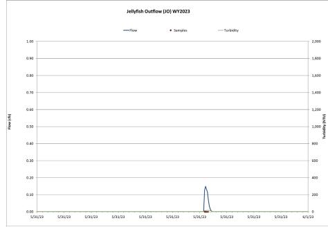
Figure 23 Hydrograph, continuous turbidity, and sample distribution at the Jellyfish Outflow for the 5/31/2023 thunderstorm event.
