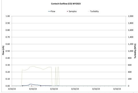
Figure 13 Hydrograph continuous turbidity, and sample distribution at the Contech Outflow for the 3/10/2023 atmospheric river rain on snow event.
