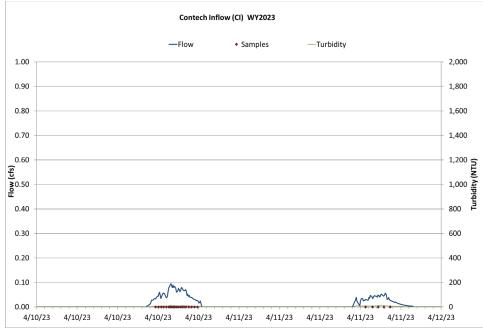
Figure 20 Hydrograph, continuous turbidity, and sample distribution at the Contech Inflow for the 4/10/2023-4/11/2023 non-event snowmelt.
