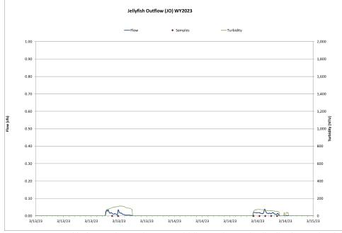
Figure 15Hydrograph, continuous turbidity, and sample distribution at the Jellyfish Outflow for the 3/13/2023 –<br/>3/14/2023 atmospheric river rain on snow event.
