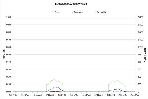
Figure 21 Hydrograph, continuous turbidity, and sample distribution at the Contech Outflow for the 4/10/2023-4/11/2023 non-event snowmelt.
