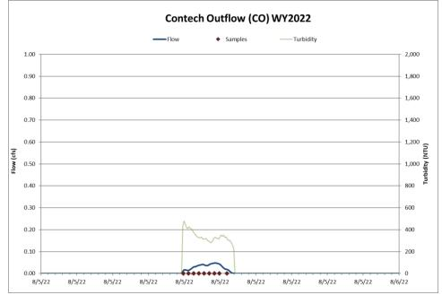
Figure 14 Hydrograph continuous turbidity, and sample distribution at the Contech Outflow for the 8/5/2022 thunderstorm event.
