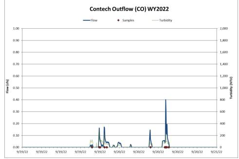
Figure 22 Hydrograph, continuous turbidity, and sample distribution at the Contech Outflow for the 9/19/2022-9/21/2022 rain event.
