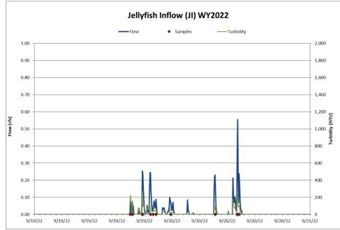
Figure 19 Hydrograph, continuous turbidity, and sample distribution at the Jellyfish Inflow for the 9/19/2022-9/21/2022 rain event.
