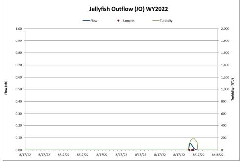
Figure 16 Hydrograph, continuous turbidity, and sample distribution at the Jellyfish Outflow for the 8/17/2022 thunderstorm event.
