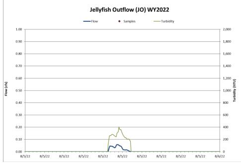
Figure 12 Hydrograph and continuous turbidity at the Jellyfish Outflow for the 8/5/2022 thunderstorm event. Samples failed during this event at Jellyfish Outflow.
