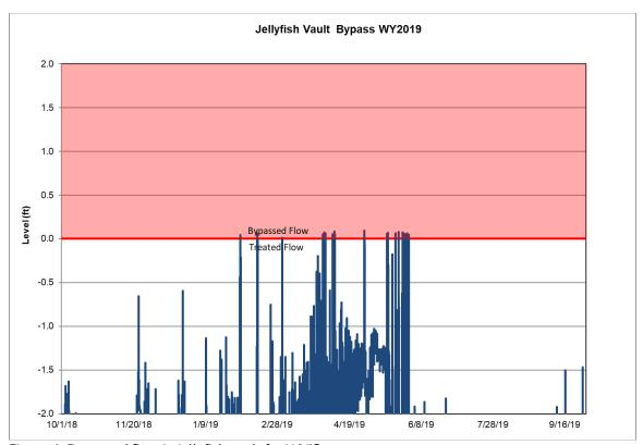
Figure 6: Bypassed flow in Jellyfish vault for WY19.
