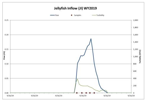
Figure 10: Hydrograph, continuous turbidity and sample distribution at the Jellyfish Inflow for the 9/16/19 rain event.
