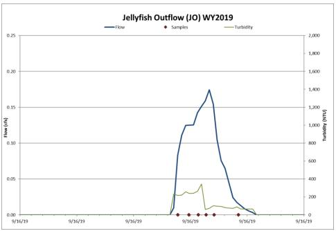
Figure 11: Hydrograph, continuous turbidity and sample distribution at the Jellyfish Outflow for the 9/16/19 rain event.
