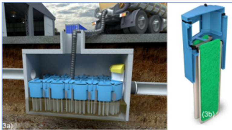
Figure A-10: Schematic of a filter for very fine particles. Washington State TAPE https://ecology.wa.gov/ .
