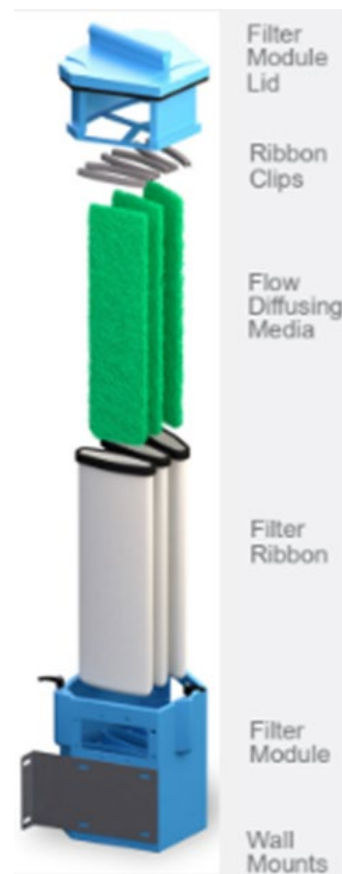
Figure A-10: Schematic of a filter for very fine particles. Washington State TAPE https://ecology.wa.gov/ .
