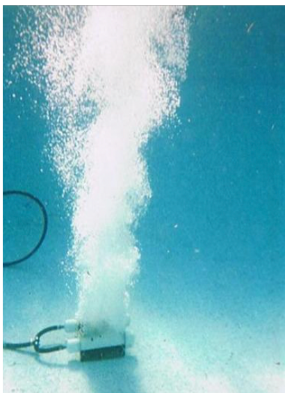
Diffused aeration device Image from www.aquaticbiologists.com
