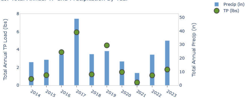
Figure 84 Total annual TP load and precipitation by year for Contech MFS Inflow WY14-WY23.
