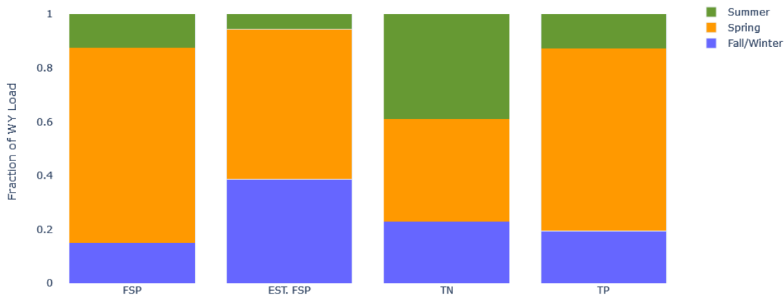
Figure 21 Seasonal load as a fraction of the water year load at the Contech MFS outflow, WY23. The first FSP column represents the FSP load calculated using event mean concentrations and the second FSP column (EST. FSP) represents the FSP load estimated using continuous turbidity data.
