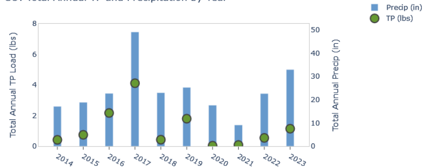
Figure 85 Total annual TP load and precipitation by year for Contech MFS Outflow WY14-WY23.
