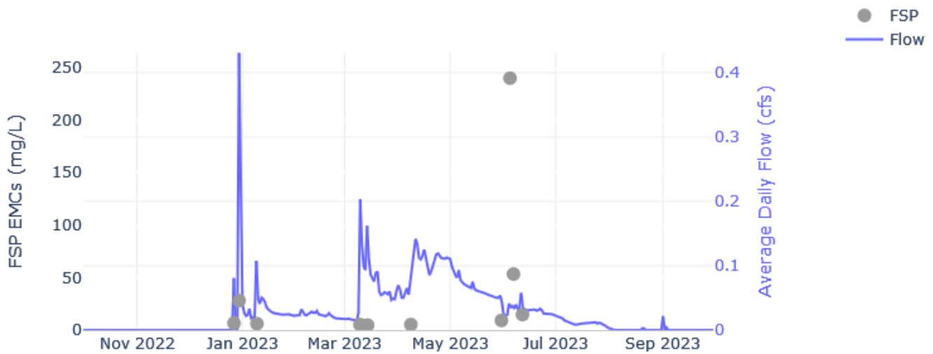
Figure 31 Daily flow and FSP EMC summary at the Elks Club catchment outfall, WY23.
