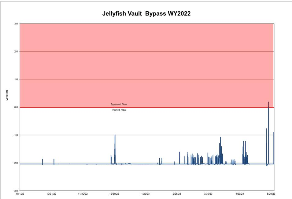
Figure 5 Bypassed flow in the Jellyfish vault for WY23.
