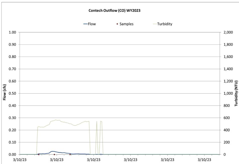
Figure 13 Hydrograph continuous turbidity, and sample distribution at the Contech Outflow for the 3/10/2023 atmospheric river rain on snow event.
