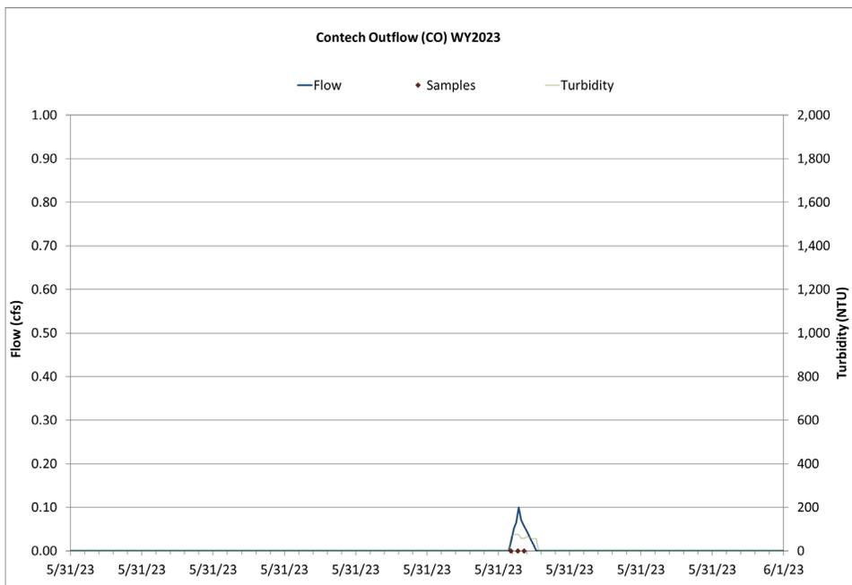
Figure 25 Hydrograph, continuous turbidity, and sample distribution at the Contech Outflow for the 5/31/2023 thunderstorm event.
