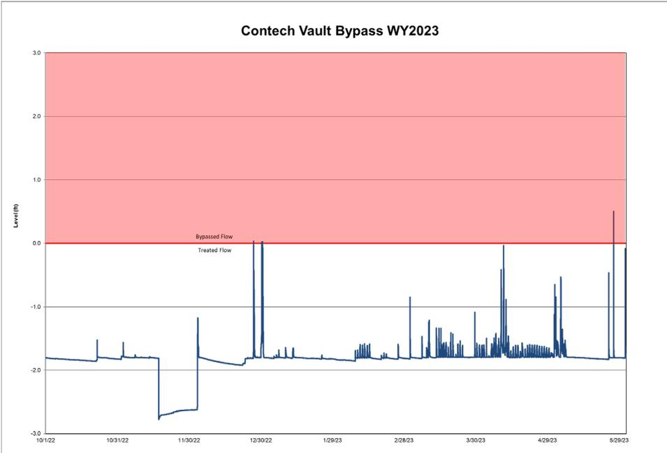
Figure 4 Bypassed flow in the Contech MFS vault for WY23.
