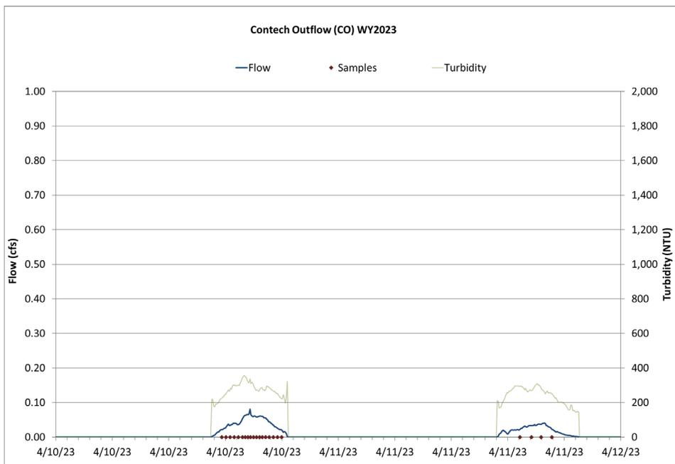
Figure 21 Hydrograph, continuous turbidity, and sample distribution at the Contech Outflow for the 4/10/2023-4/11/2023 non-event snowmelt.
