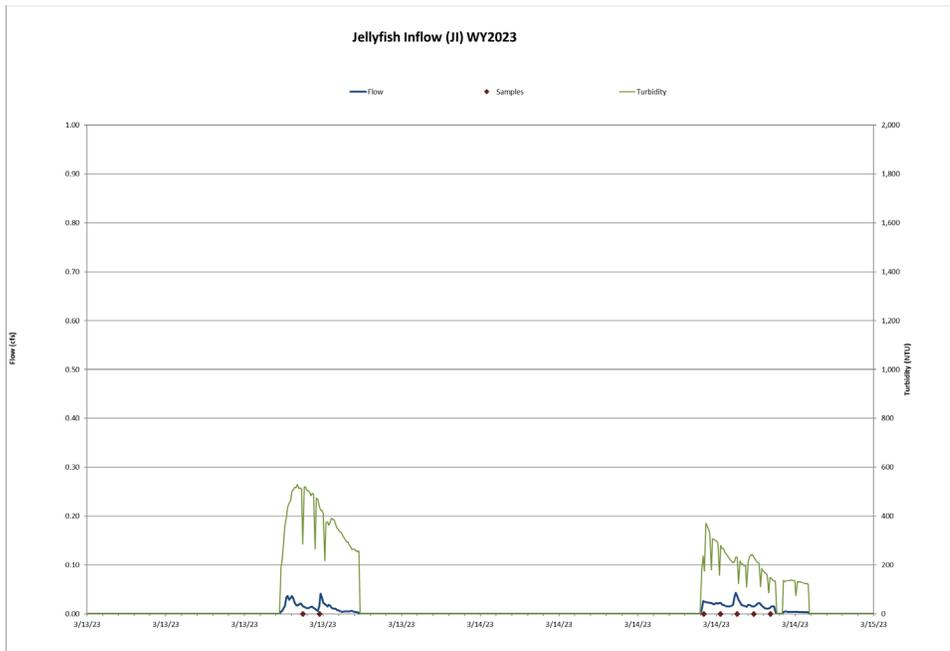
Figure 14 Hydrograph, continuous turbidity, and sample distribution at the Jellyfish Inflow for the 3/13/2023 – 3/14/2023 atmospheric river rain on snow event.
