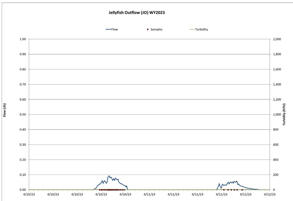
Figure 19 Hydrograph, continuous turbidity, and sample distribution at the Jellyfish Outflow for the 4/10/2023-4/11/2023 non-event snowmelt.
