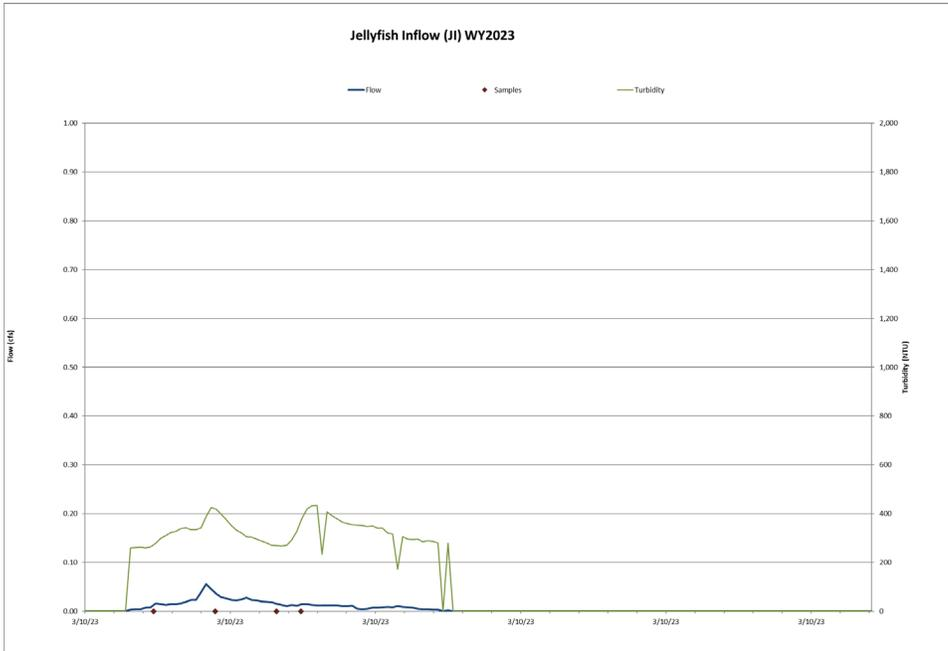
Figure 10 Hydrograph, continuous turbidity, and sample distribution at the Jellyfish Inflow for the 3/10/2023 atmospheric river rain on snow event.
