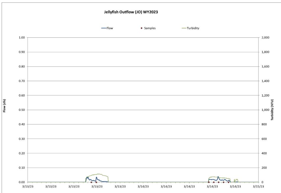
Figure 15 Hydrograph, continuous turbidity, and sample distribution at the Jellyfish Outflow for the 3/13/2023 – 3/14/2023 atmospheric river rain on snow event.
