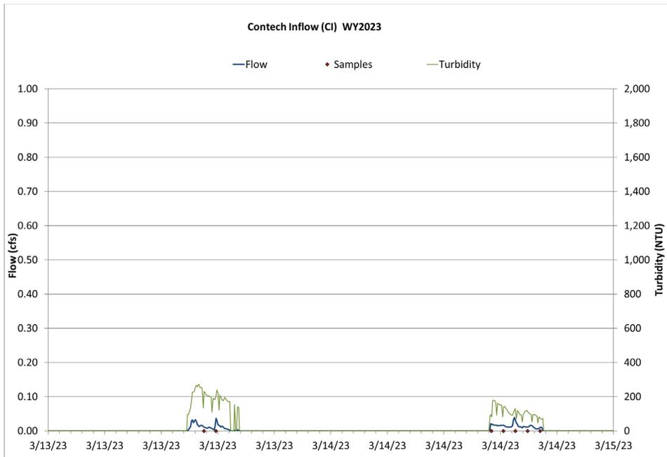
Figure 16 Hydrograph, continuous turbidity, and sample distribution at the Contech Inflow for the 3/13/2023 – 3/14/2023 atmospheric river rain on snow event.
