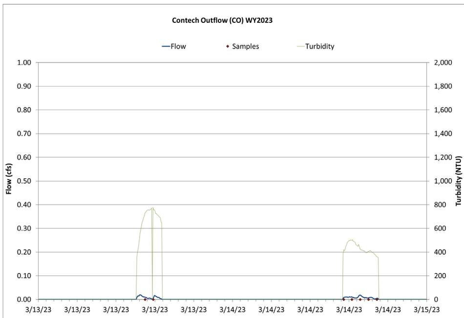
Figure 17 Hydrograph, continuous turbidity, and sample distribution at the Contech Outflow for the 3/13/2023 – 3/14/2023 atmospheric river rain on snow event.
