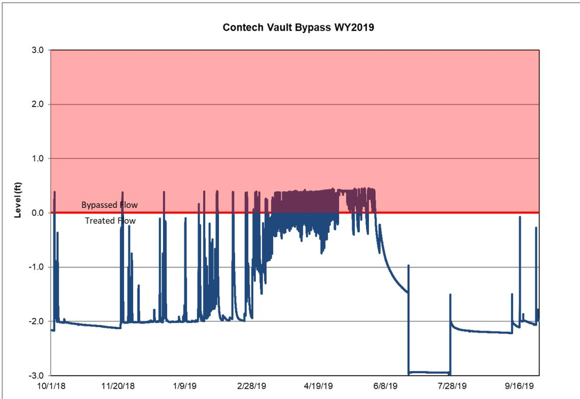
Figure 5: Bypassed flow in Contech MFS vault for WY19.
