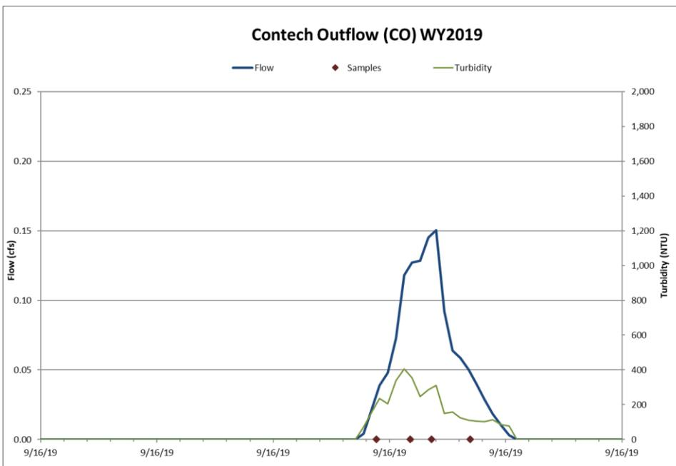
Figure 9: Hydrograph, continuous turbidity and sample distribution at the Contech MFS Outflow for the 9/16/19 rain event.
