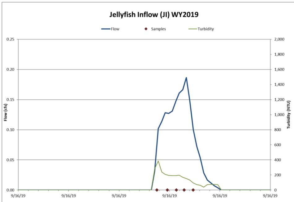
Figure 10: Hydrograph, continuous turbidity and sample distribution at the Jellyfish Inflow for the 9/16/19 rain event.
