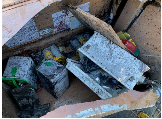
Figure 2 Inside of Jobbox, batteries and dataloggers covered in battery acid.
