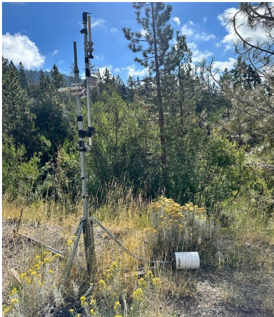
Figure 3 Meteorological station with tipping bucket ripped down.
