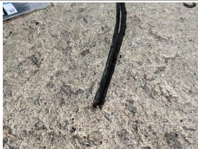
Figure 3 Severed pressure transducer cord discovered on September 14, 2022.
