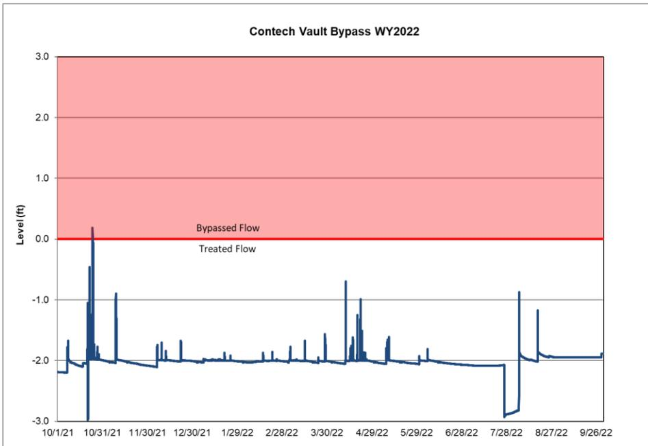
Figure 5 Bypassed flow in the Contech MFS vault for WY22.
