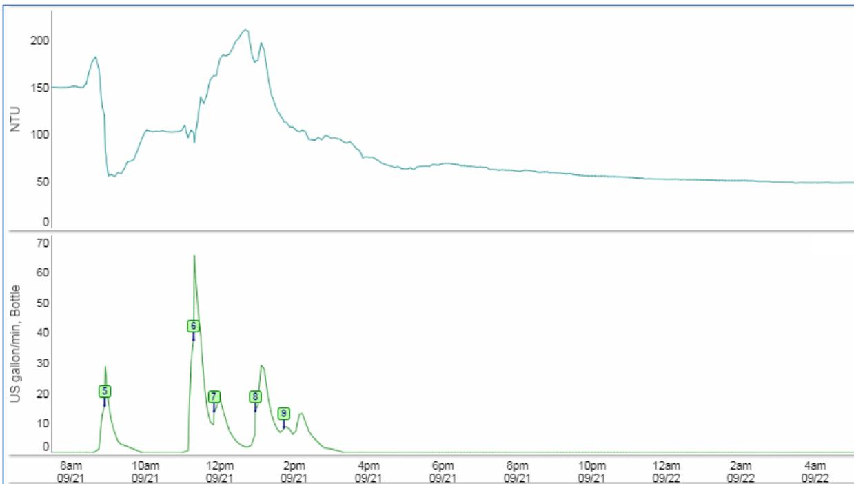
Figure 14: Hydrograph, continuous turbidity and sample distribution at the Jellyfish Outflow for the 9/21/17 thunderstorm event.
