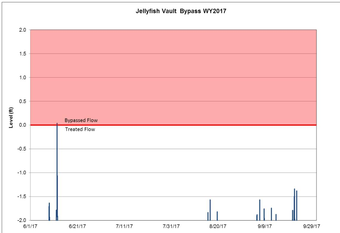
Figure 6: Bypassed flow in Jellyfish vault, summer WY17.
