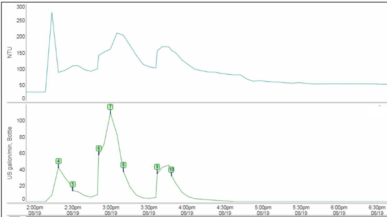
Figure 10: Hydrograph, continuous turbidity and sample distribution at the Jellyfish Outflow for the 8/19/17 thunderstorm event.
