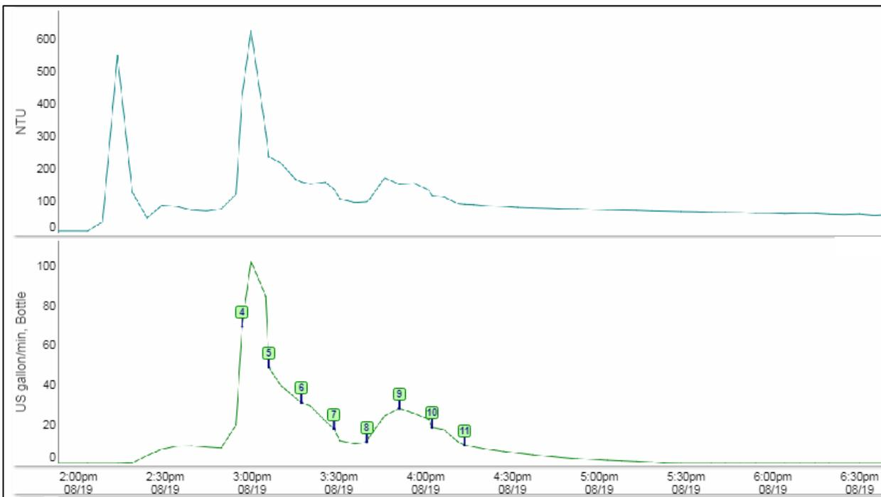
Figure 8: Hydrograph, continuous turbidity and sample distribution at the Contech MFS Outflow for the 8/19/17 thunderstorm event.
