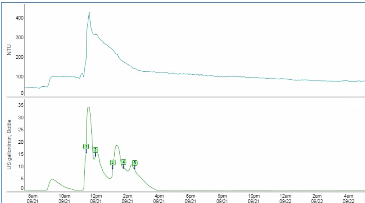
Figure 12: Hydrograph, continuous turbidity and sample distribution at the Contech MFS Outflow for the 9/21/17 thunderstorm event.
