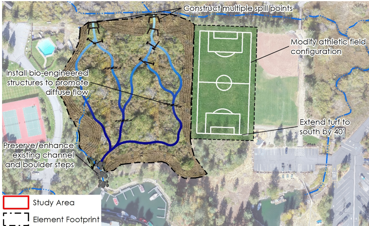
Figure 23. Design Element 2B: Athletic field area partial restoration with athletic field reconfiguration. The shaded blue areas are schematic in nature to illustrate spreading of water as a design intent. This should not be interpreted as design of new channels.
