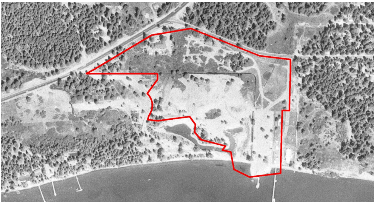
Figure 13. Aerial photograph from 1969 (Study Area outlined in red). Most disturbance to the Polaris wetland complex occurred in the mid-1950s through 1960s. The campground, boat ramp, coast guard station, and Star Harbor development were built during this time. An artificial harbor was excavated and fill placed in the present-day athletic field area. The east-west ditch was constructed to route surface water around the fill.
